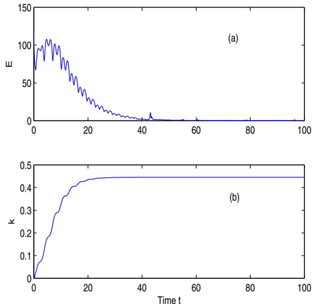
Fig. 1: (a) and (b) show the temporal evolution of the absolute synchronization error  $E = \sum_{i=1}^N [|x_i - x| + |y_i - y| + |z_i - z|]$  and the adaptive coupling strength  $k$  in system (6), respectively, where the pristine network structure is the simple cycle configuration, *i.e.*,  $n = 1$ .
