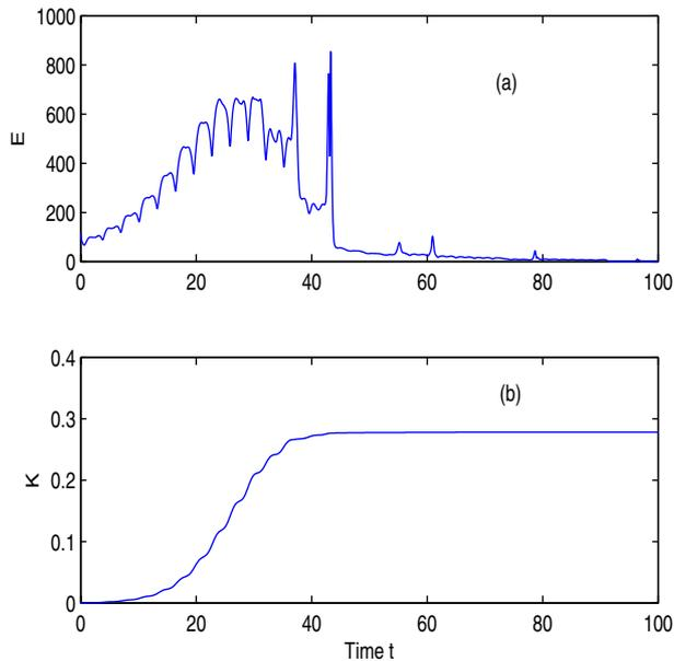
Fig. 3: (a) and (b) show the temporal evolution of the absolute synchronization error  $E$  and the average coupling strength  $K = \frac{1}{N} \sum_{i=1}^N k_i$  in the weighted coupling system (7), respectively, where the connectivity structure in its pristine network is same as that in fig. 1.
